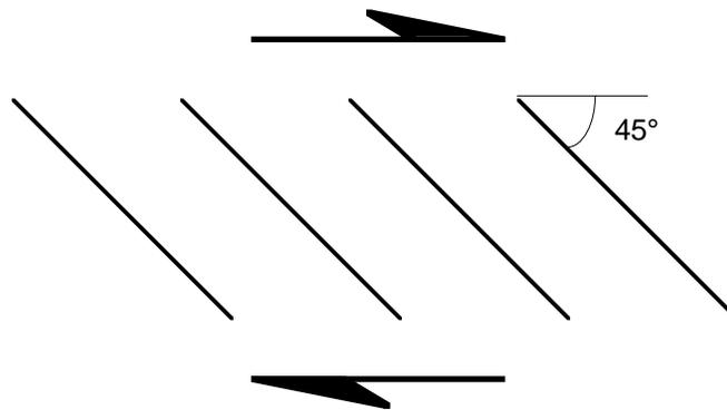
These cracks can serve to break out blocks which subsequently rotate in the shear zone, domino-style:
