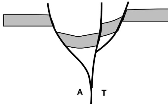
Extensional basins formed along strike-slip faults are called “pull-apart” basins.
