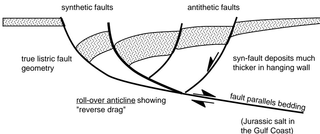
The key to recognizing growth structures is that sediments of the same age are much thicker on the hanging wall than they are on the footwall. This means that the fault was moving while the sediments accumulated preferentially in the depression made by the fault.
