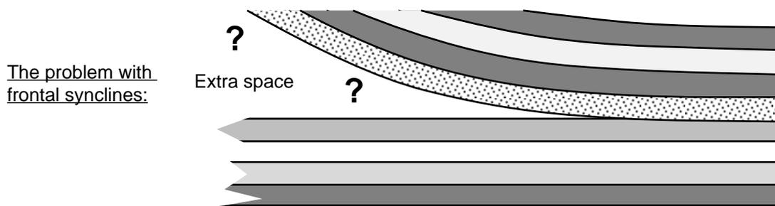
The problematical space is triangular in shape so it is known as a **triangle zone**. The solution to this dilemma of frontal synclines is to fill the space with a type of duplex:
