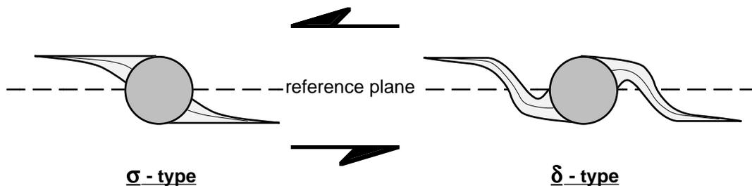
In the  $\sigma$ -type, the median line of the recrystallizing tails does not cross the reference plane, whereas in the  $\delta$ -type, the median line of the recrystallizing tails does cross the reference plane. The ideal conditions for the development of asymmetric porphyroclasts are:
