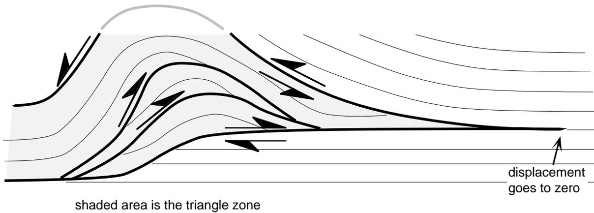
This duplex differs from the ones that we discussed above, in that the roof thrust has the opposite sense of shear than the floor thrust, whereas in "normal" duplexes they have the same sense of shear. For this reason, triangle zones have sometimes been referred to as **passive roof duplexes**. You can best visualize the kinematics of this structure by imagining driving a wedge into a pack of cards:
