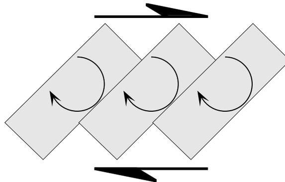
Note that the faults between the blocks have the opposite sense of shear than the shear zone itself.
