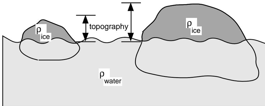
The way to get more topography is to make the ice (or wood) thicker. The topography itself and the ratio of the part of the iceberg above and below water is a direct function of the ratio of the densities of ice and water. This basic principle is known as isostasy.
