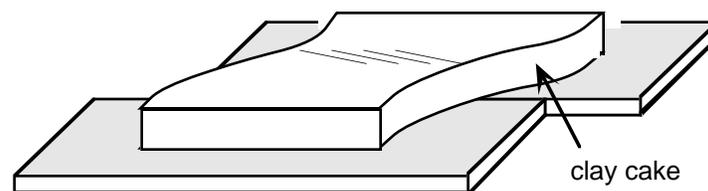
Much of our basic understanding of the array of structures that develop during parallel strike-slip faulting comes from experiments with clay cakes deformed in shear, as in the picture, above. These experiments show that strike-slip is a two stage process involving
