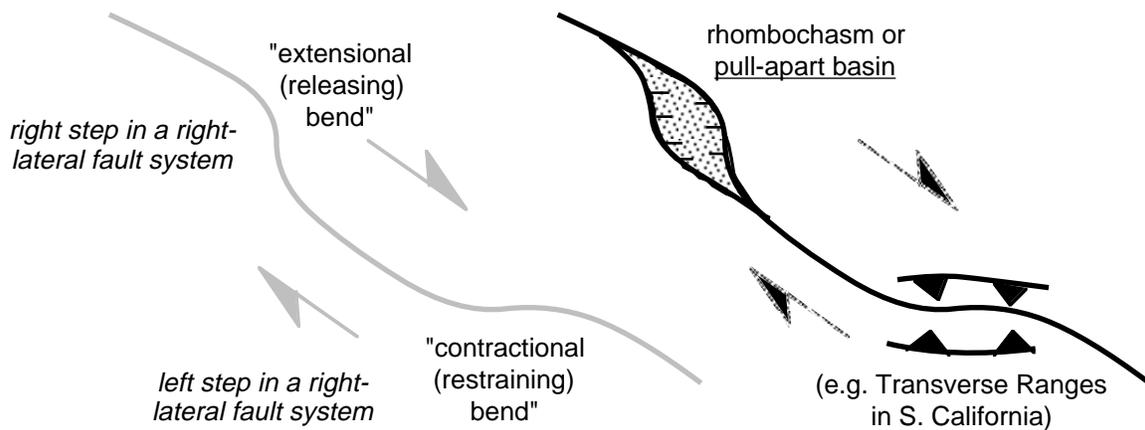
Restraining or releasing bends can be the site of formation of strike-slip duplexes, in which the faults can either be contractional or extensional, respectively. Extensional or contractional structures can also be concentrated at the overlaps in an echelon strike-slip fault segments:
