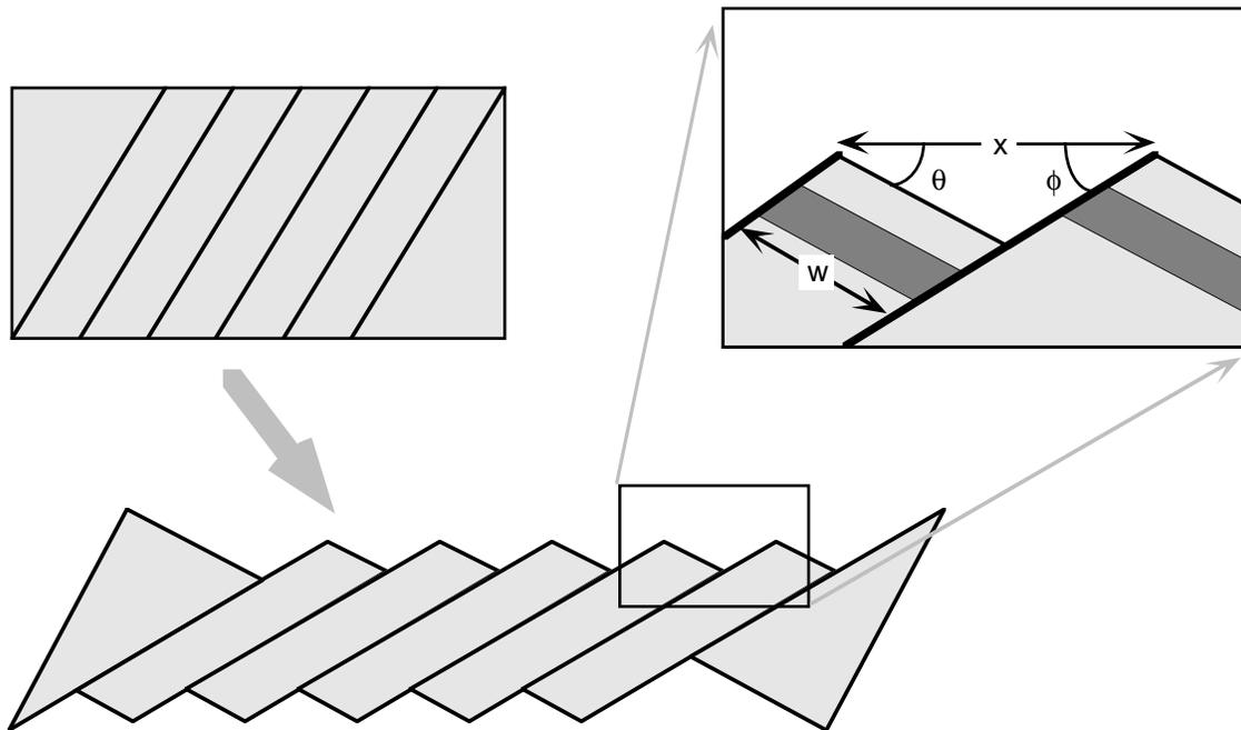
If you know the dip of the rotated bedding and the dip of the fault, you can calculate the horizontal extension assuming a domino model from the following equation (from Thompson, 1960):
