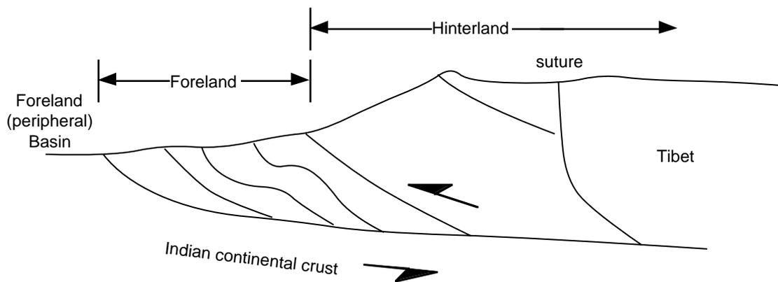
The Himalayan type is sometimes called a synthetic thrust belt because the sense of shear is the same as the plate margin that preceded it. At this point, we need to introduce two additional terms:
