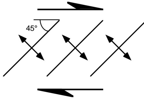
The folds in the shear zone form initially at  $45^\circ$  to the shear zone walls, but then rotate to smaller angles.
